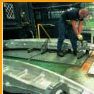
Left The C-17 military transporter is an important programme for GKN Aerospace Services' St Louis plant. Ervin Mayhew adds clamping provisions to a C-17 main landing gear in preparation for machining on a multi-spindle gantry profile.
